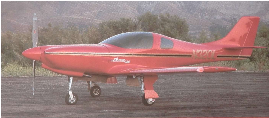
Lancair 320, 2 Plätze, 160 PS, Cruise 390 km/h, Range 2'330 km, 8 l/100 km «Until Ferrari builds an airplane, this is it»
